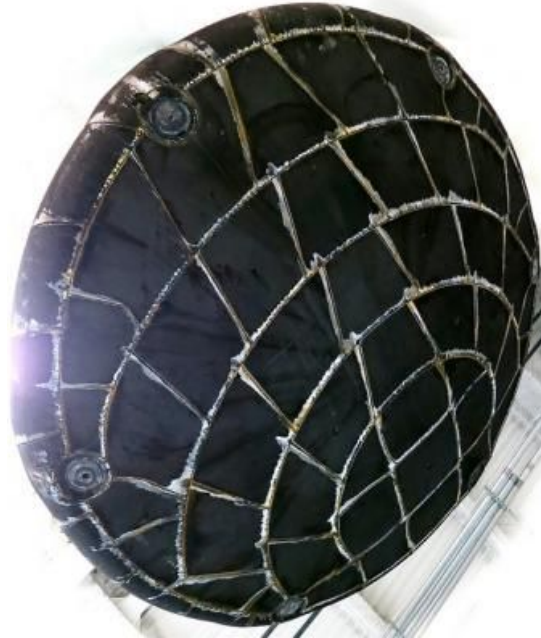
SpaceX's Dragon 1 capsule heat shield-holes indicated to take sample core testing
