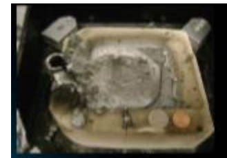
Small casting of molten ferrosilicon (lower layer) and molten oxide of lunar composition (top layer) withdrawn by counter-gravity suction at 1600°C from reactor furnace
