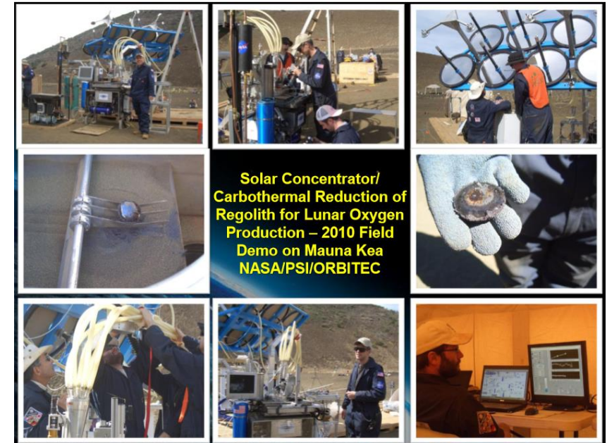
2010 (ORBITEC/PSI) Field Test 1000 kg O 2 /y scale
