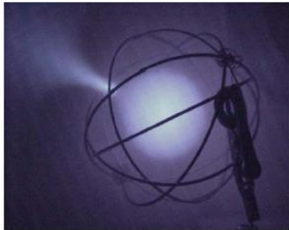
Figure 2. The IEC plasma during microwave irradiation. Note the plasma shrinkage relative to the grid structure as seen Figure 1.
